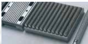
Broach for machining steering racks.
