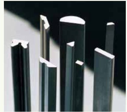
High-grade special steel pre-shaped into forms that approach the final product.
