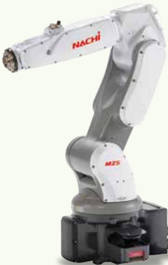
Collision-free, collaborative robot Detects proximity of people via internal arm sensor. Stops operating before contact and resumes work when the person steps away, achieving both safety and productivity.
