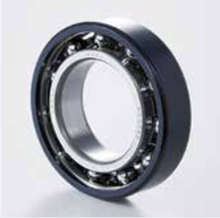
Plastic insert Bearings Integrated molding with plastic for superior isolation of the outer and inner rings prevents electrolytic corrosion from electrical current reaching the interior of the bearing.
