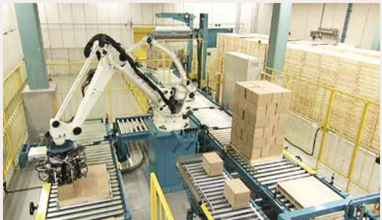
Palletizing Robot LPA180 Enables high-speed/high-precision palletization of cardboard boxes, bags, bottles, and metal products.
