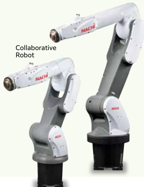
Collision-free, collaborative robot Detects proximity of people via internal arm sensor. Stops operating before contact and resumes work when the person steps away, achieving both safety and productivity.
