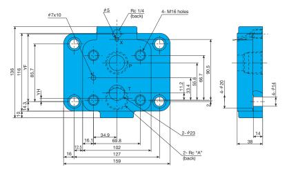
Attach a plug when the vent (X) port is not used.
