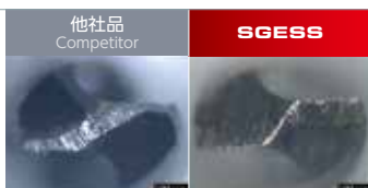
定数での摩耗比較 \phi 0.99 Comparison of tool wear
